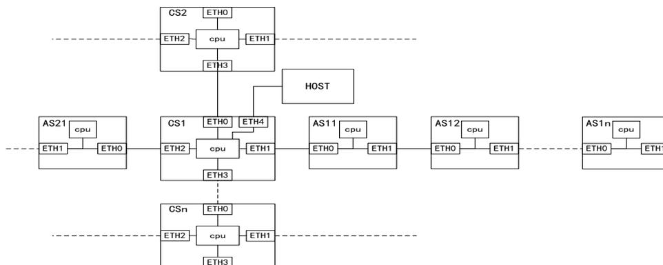
Fig. 1 3D exploration relay network topology
