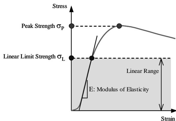
**Fig. 2** Typical stress-strain curve of hardfill
