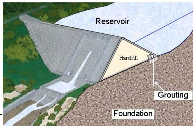
**Fig.3** Sketch of a hardfill dam
