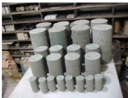
**Fig.5** Test specimen of hardfill material
