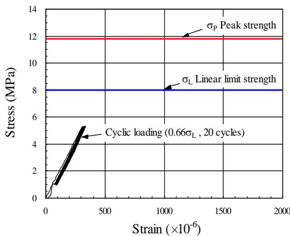
**Fig.8** Stress-strain curve (case 3)
