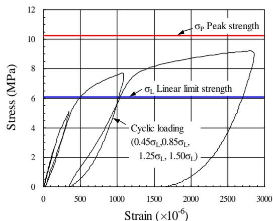
**Fig.9** Stress-strain curve (case 4)
