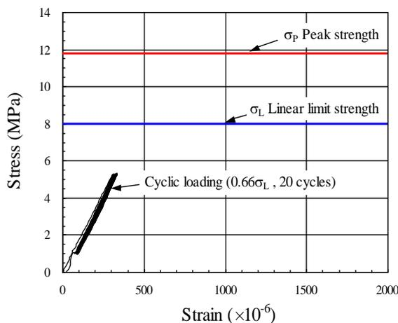
**Fig.8** Stress-strain curve (case 3)
