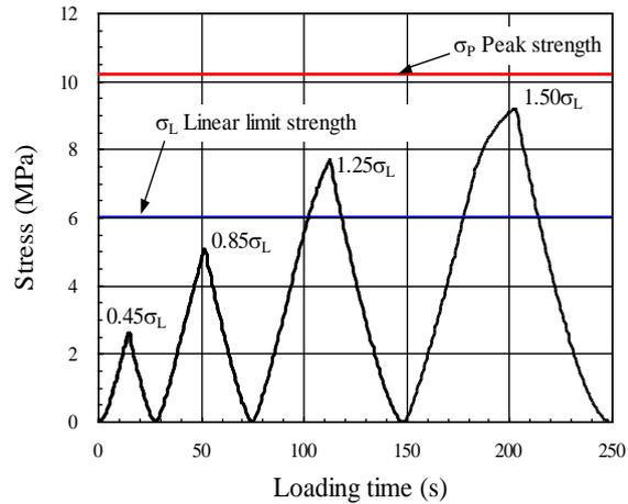
**Fig.7** Loading pattern (case 4)
