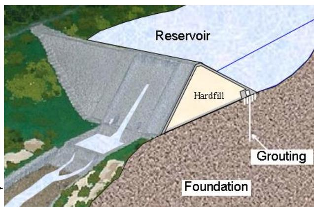
**Fig.3** Sketch of a hardfill dam
