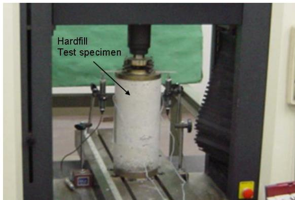
**Fig.4** Uniaxial compression test of hardfill material
