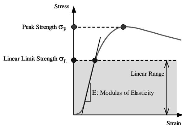
**Fig. 2** Typical stress-strain curve of hardfill
