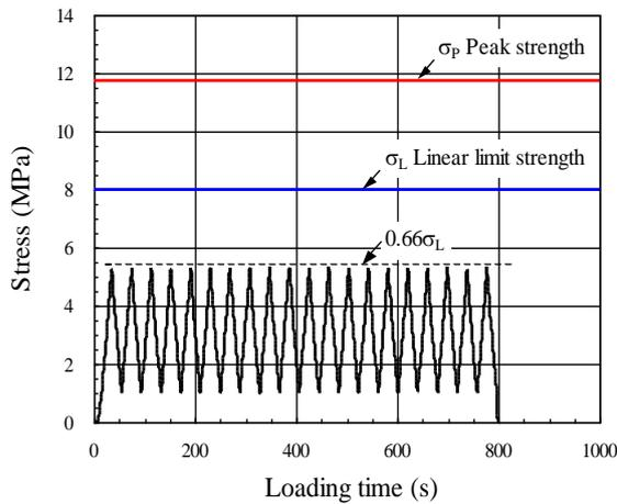
**Fig.6** Loading pattern (case 3)
