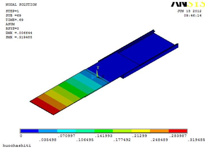
Fig.5 1st step of the Von Mises stress distribution
