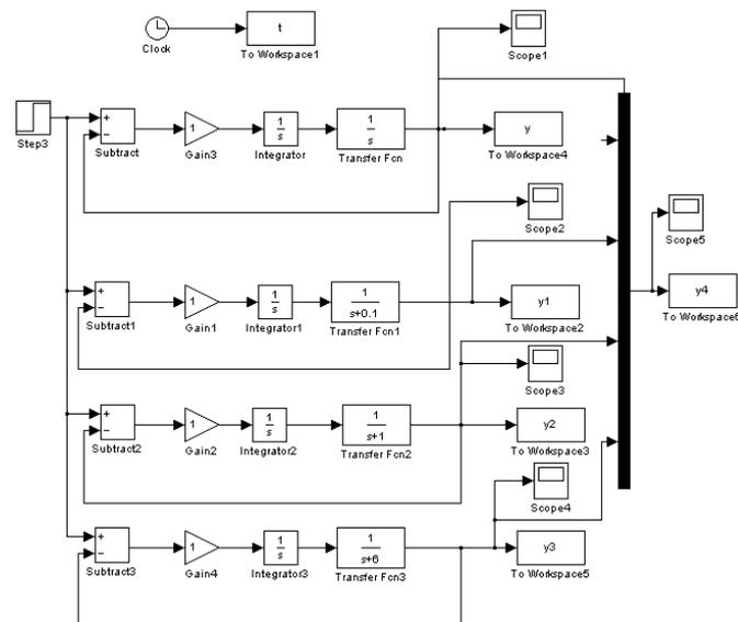
Fig.10 Simulation controller structure
