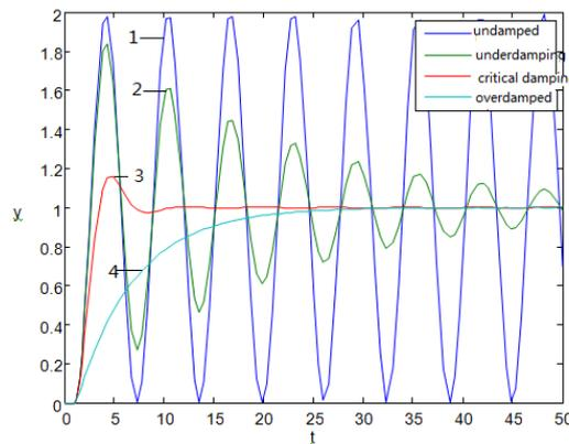
1- undamped condition, 2- under-damping condition,3- critical damping condition, 4- over-damped condition.
