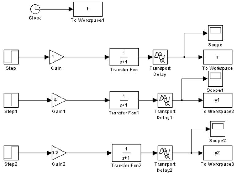
Fig.2 Simulation controller structure
