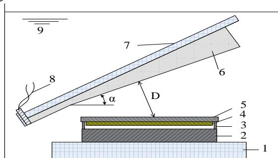
Fig.4 The method of regulated underwater shockwave
