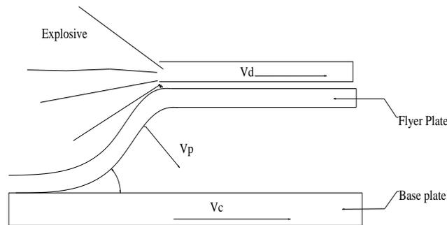
Fig.1 Explosive welding parameters
