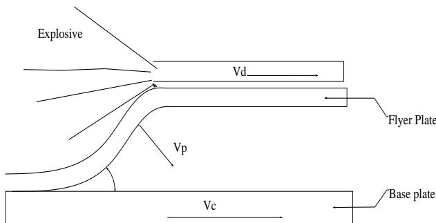
Fig.1 Explosive welding parameters
