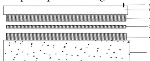
Fig.3 Schematic diagram of Multi-layer explosive welding set-up
