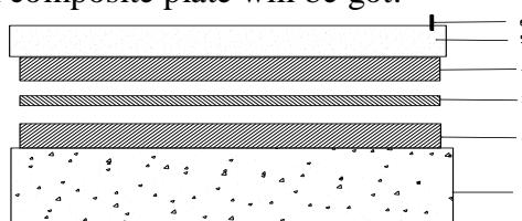
Fig.3 Schematic diagram of Multi-layer explosive welding set-up
