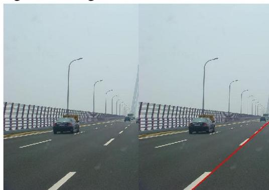
Fig.4 Result of the right lane detection
