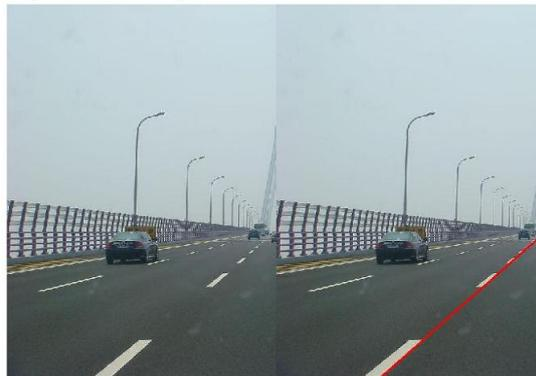
Fig.4 Result of the right lane detection
