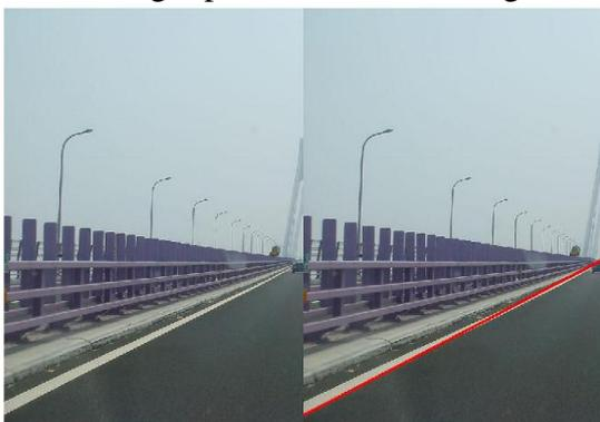
Fig.3 Result of the left lane detection
