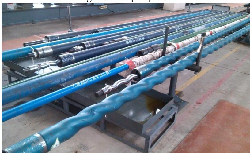
Fig.2. The practical screw pump of our production
