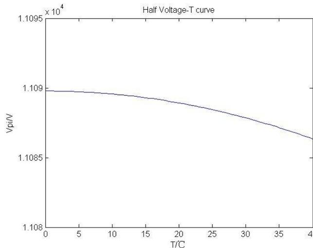
Figure 1. Curve of drift about half-wave voltage with temperature
