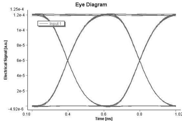
Figure 5. Output eye-diagram of EOM based on auto control of bias voltage
