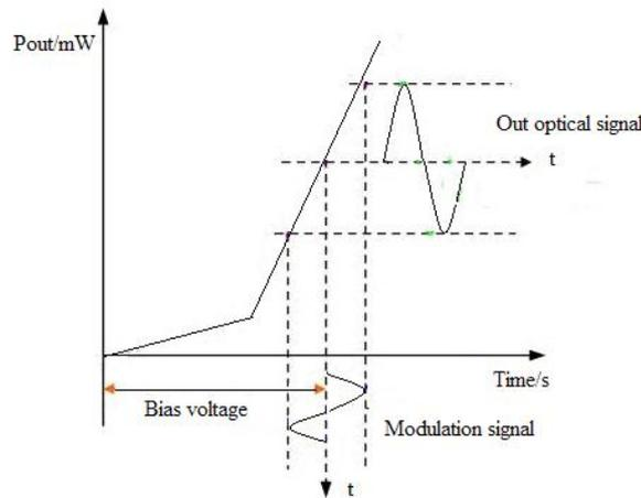
Figure 2. Curve of modulation characteristic about EOM
