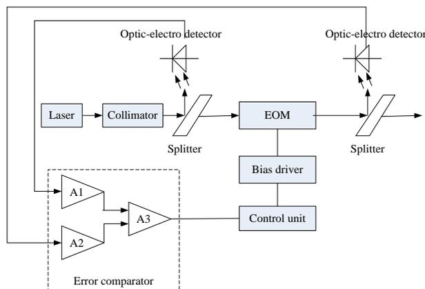
Figure 3. Auto control circuit of bias voltage
