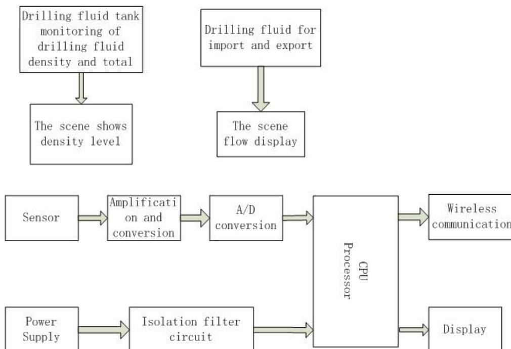
Fig.1 Well control the bop early warning monitoring system principle
