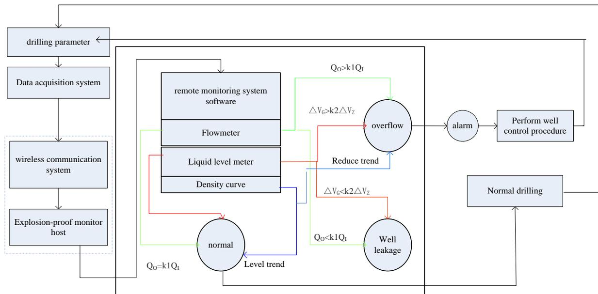
Fig.2 warning system program block diagram
