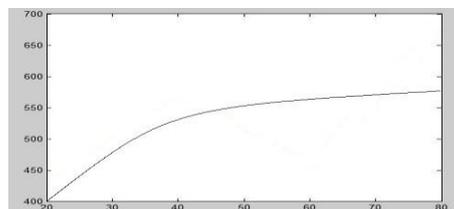
Figure 2. Kalman filter effect of boiler internal temperature sampling signal
