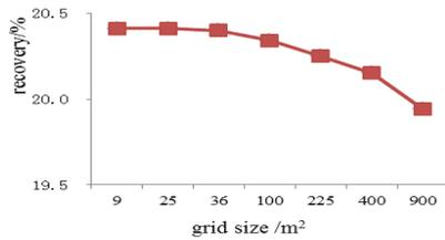
Fig.1: The relation curve between the grid size and recovery degree
