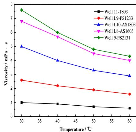
Figure 4. Viscosity-temperature curve. The polymer concentration of these five produced wells as follows: Well 11-1803, 72 mg/L; Well L9-PS1233, 473 mg/L; Well L10-AS1803, 557 mg/L; Well L8-AS1603, 1222 mg/L; Well 9-PS2131, 1032 mg/L.
