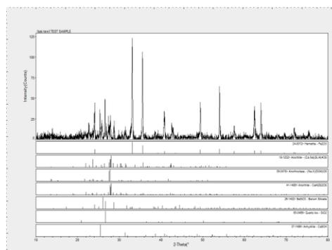
Figure 3. XRD of the scale-like mud
