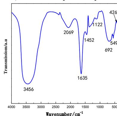
Figure 1. FT-IR spectrum of the suspended solids in the oil-water phase
