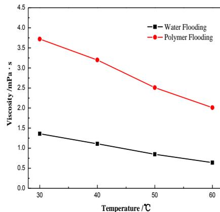
Figure 5. Viscosity-temperature curve for both water flooding and polymer flooding
