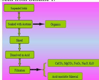
Scheme 1. The flow diagram for analyzing suspended solids
