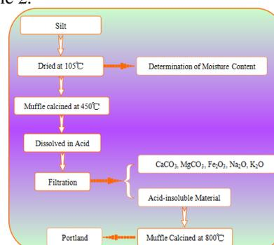
Scheme 2. The flow diagram for analyzing the silt
