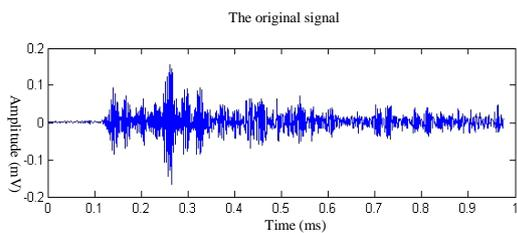
Figure 5. Original signal waveform after decomposition and reconstruction
