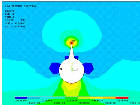
(b) Current distribution of defect model at 1000A
