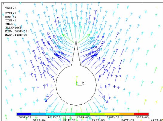
(b) Electromagnetic force vector of defect model at 1000A
