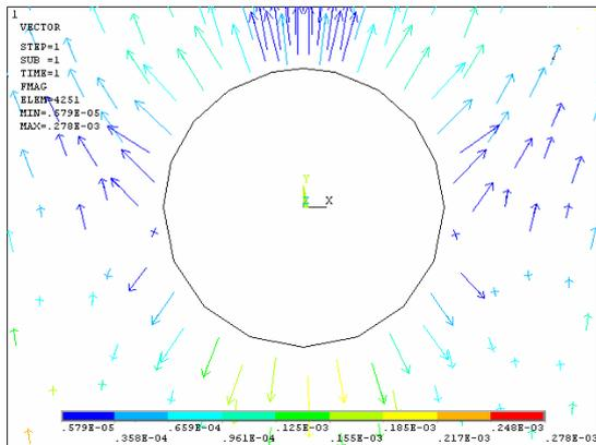
(a) Electromagnetic force vector of intact model at 1000A
