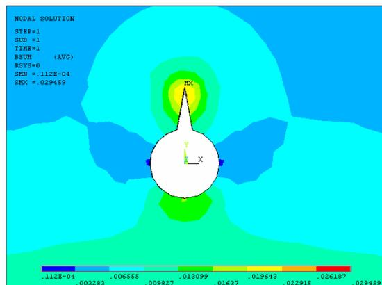
(b) Magnetic flux density of defect model at 1000A
