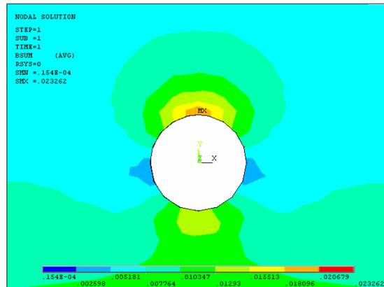
(a) Magnetic flux density of intact model at 1000A
