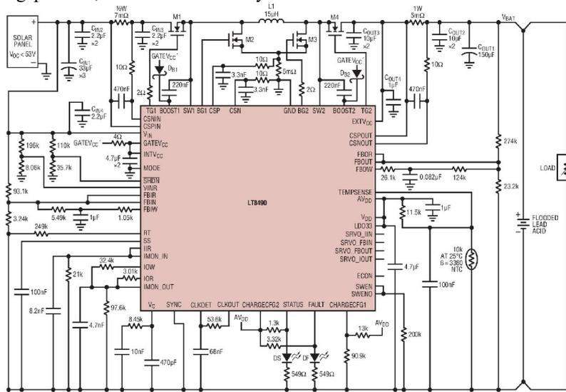
Figure 3. Battery charging circuit model
