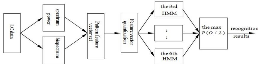
Figure 1 Multi-Feature Fusion with Multi- Mode HMM Mode Recognition
