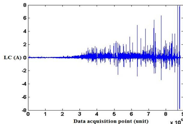
Figure 3 Leakage Current Waveform (ESDD =  $0.15 \text{ mg/cm}^2$ )
