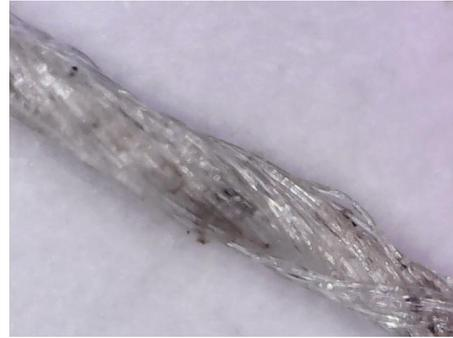
Fig.2 double coated yarn of 36Nm linen yarn after scouring drying and shaping.
