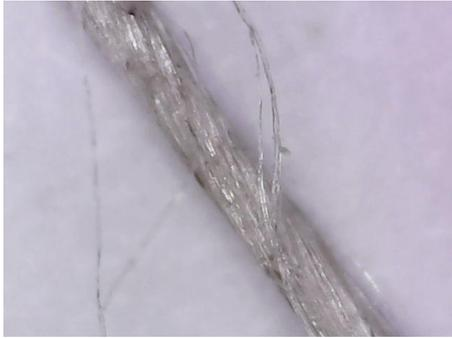
Fig.1 36Nm linen yarn after scouring
