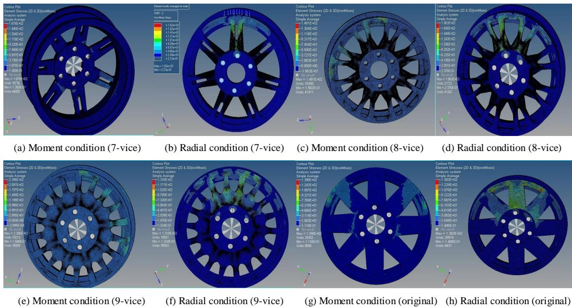
Figure 9 The stress distributions of each wheel hub in moment and radial conditions
