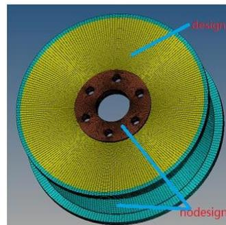
Figure 2 Design and non-design areas in the finite element concept model
