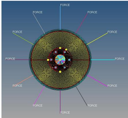
Figure 3 Simulation of the hub’s moment condition
