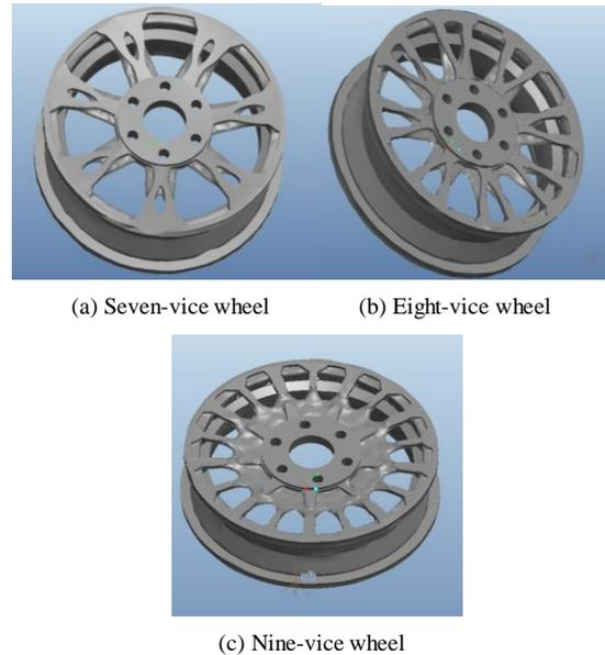
Figure 7 3D geometric model of wheel hub after introducing
