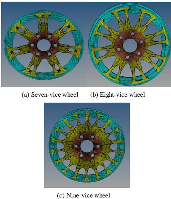
Figure 6 The three structure types after optimization
