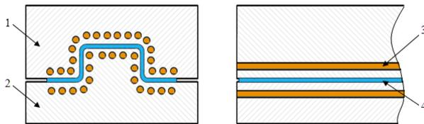
1-concave die 2-punch 3-cooling tube 4-workpiece
