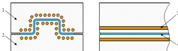
1-concave die 2-punch 3-cooling tube 4-workpiece
