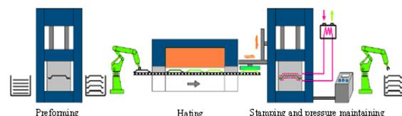
Fig. 1 Schematic diagram of hot stamping
