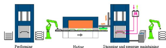
Fig. 1 Schematic diagram of hot stamping
