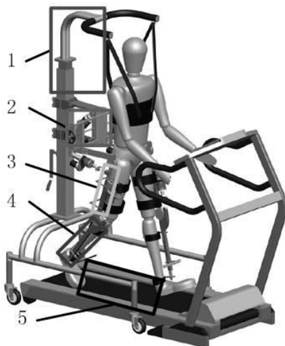
Figure 4 3D model of exoskeleton system (1- overhang weight loss frame; 2- back adjustment mechanism; 3- thigh bar, 4- crus bar; 5- treadmill).
