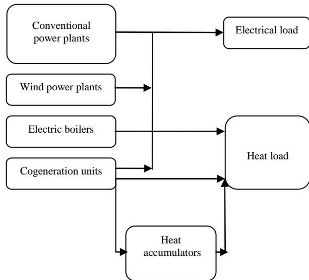
Figure 1 Diagram of accommodating wind power curtailment by combined heat and power plant
