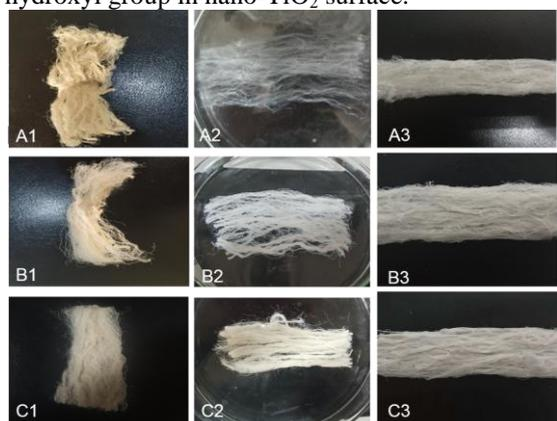
Figure 6 Appearance change of the fiber. (1: normal fiber; 2: fiber in water; 3: dried fiber. A. Fiber-1; B. Fiber-2; C. Fiber-3.)
