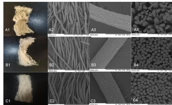
Figure 2 Digital photo and electron micrograph of fibers (1: digital photo; 2:SEM of ×100; 3:SEM of ×1000; 4: SEM of ×200; 2,3: the surface; 4: the cross-section. A. Fiber-1; B. Fiber-2; C. Fiber-3.)
