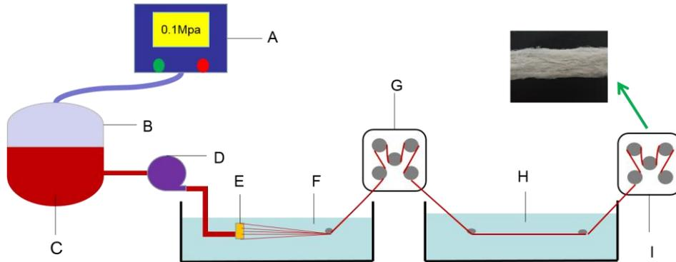
Figure 1 Process diagram showing the custom-made device used for spinning (A. air compressor; B. dope storage cylinder; C. spinning dope; D. metering pump; E. spinneret; F. coagulation bath; G. roller (I); H. stretch bath; I. roller (II).)
