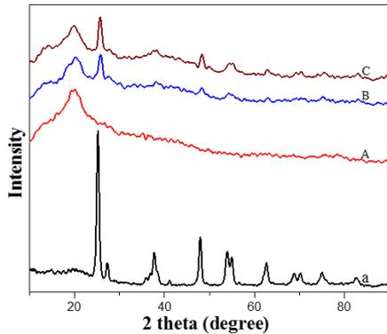
Figure 3 X-ray diffraction spectra. (a. nano-TiO<sub>2</sub> powder; A. Fiber-1; B. Fiber-2; C. Fiber-3.)
