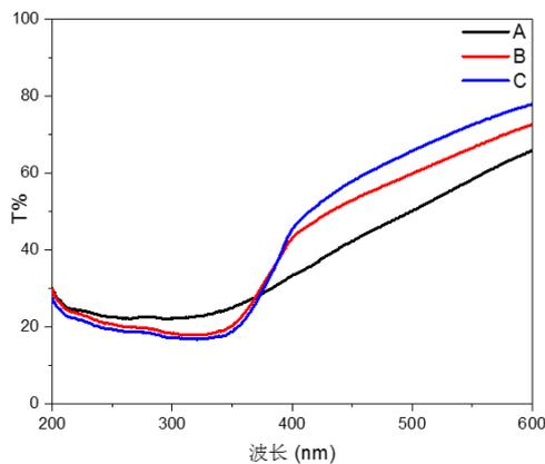
Figure 4 UV-transmittance curve. (A. Fiber-1; B. Fiber-2; C. Fiber-3.)
