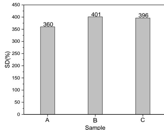
Figure 5. Water absorption ratio of the fiber. (A. Fiber-1; B. Fiber-2; C. Fiber-3.)
