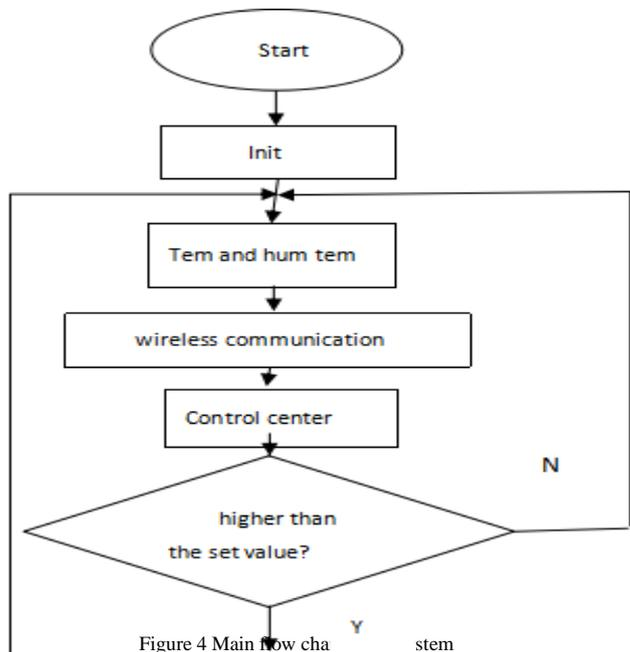
After the system module works normally, continues to collect temperature and humidity data in the environment, and sends the collected data to the STM CPU for processing. Because the monitoring environment is not strict with the data requirements, the data collected in this design only need to read the integer part, and the decimal part can be used after the system upgrade.
