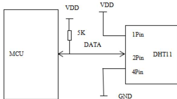
Figure 2 Typical interface connection diagram
