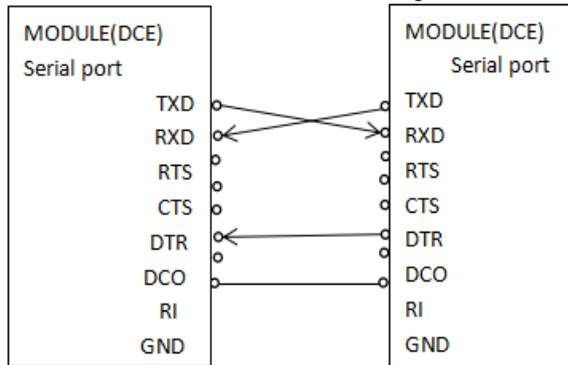
Figure 3 Non-Full Function Serial Port Mode
