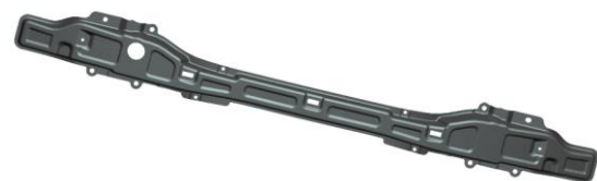
Figure.1 Model of anti-collision beam of vehicle front bumper
