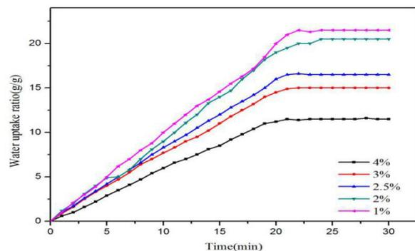
Figure 3. Relationship between water absorption ratio and absorption time of carrageenan aerogels with different carrageenan concentrations
