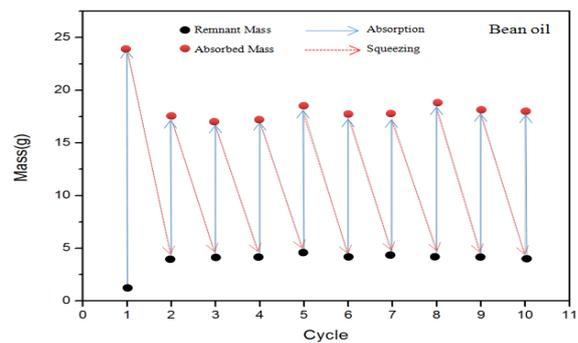
Figure 6. Repeated absorption of oil by aerogel
