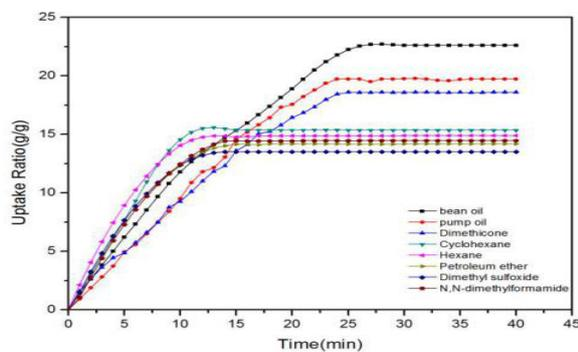
Figure 5. Absorption equilibrium curve of carrageenan aerogel in different oils/organic solvents
