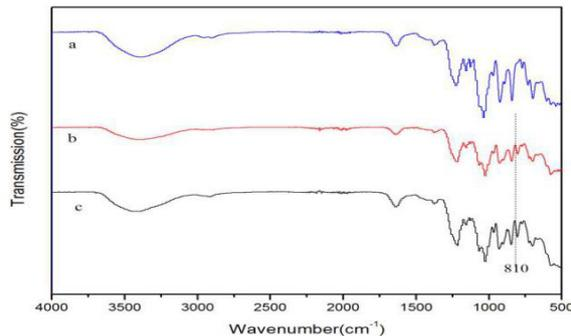
Figure1. FTIR spectrum of carrageenan((a). Commercial κ-carrageenan;(b). Carrageenan extracted from *Chondrus*; (c). Commercial ι-carrageenan)
