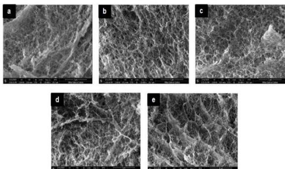
Figure 2. Scanning electron microscopy images of the fractured surface of carrageenan aerogels with concentrations of (a) 1 wt%, (b) 2 wt%, (c) 2.5wt%, (d) 3 wt%, (e) 4 wt%
