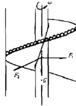
Figure 1. Movement mode of coal dust in borehole
