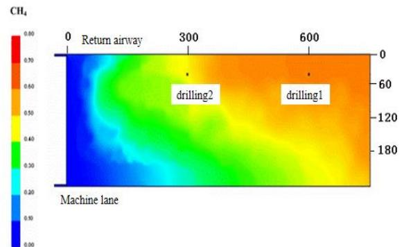
Figure 2. CFD simulation of gas distribution in goaf
