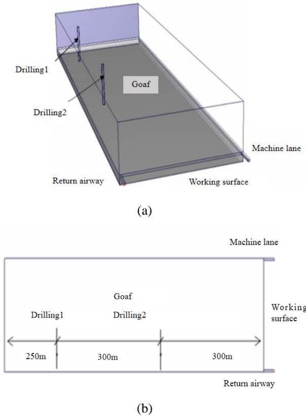
Figure 1. CFD geometric model of mining face
