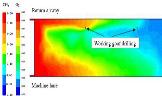
(b) Two drill holes work simultaneously
