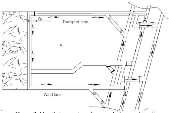
Figure 2. Ventilation system diagram during working face withdrawal
