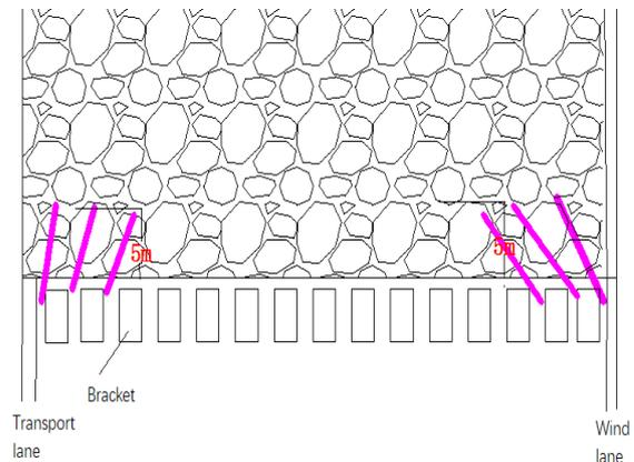
Figure 1. Schematic diagram of corner cannula grouting
