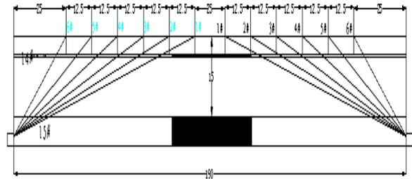
Figure 3. Fan-shaped water spray hole arrangement
