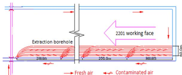
Figure 1. Schematic diagram of plane layout of long-distance large-aperture high-position fracture extraction drilling
