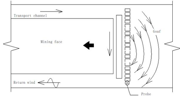
Figure 2. Single U-shaped ventilation air flow direction
