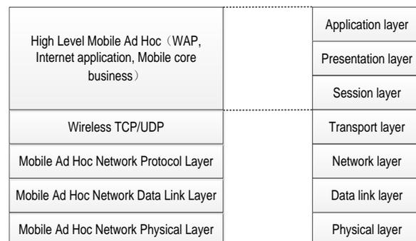
Figure 1 Different layers in Mobile Ad Hoc Network
