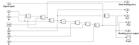
Figure 11. Braking force calculation model
