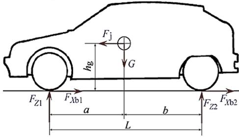
Figure 10. Braking force diagram of automobile on horizontal road
