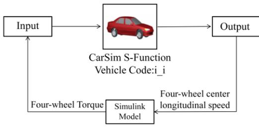
Figure 2. Co-simulation model block diagram
