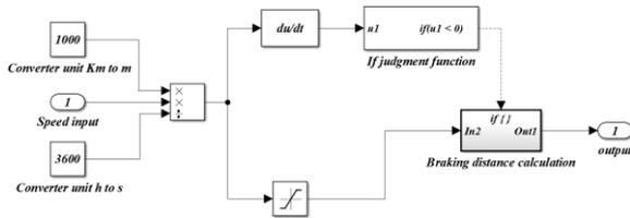
Figure 6. Braking distance calculation model
