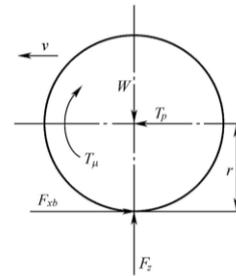
Figure 9. Wheel force diagram during automobile braking
