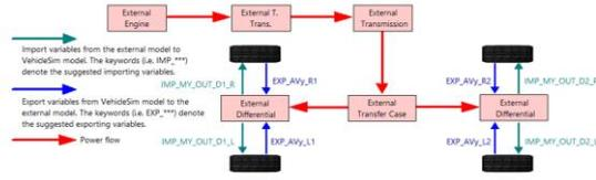
Figure 4. Diagram of power system of Carsim electric vehicle model
