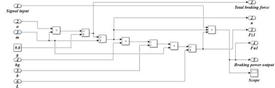
Figure 11. Braking force calculation model
