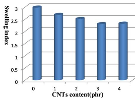
**Fig.4** Solvent resistance of NR/CNTs nanocomposites (room temperature ×4h, gasoline)
