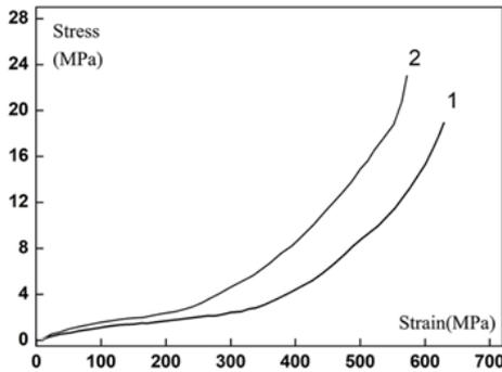
**Fig. 2** The stress-strain curve of nanocomposites when the amount of CNTs added is 0 phr and 3phr
