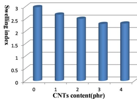
**Fig.4** Solvent resistance of NR/CNTs nanocomposites (room temperature ×4h, gasoline)
