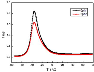
Fig.5 Comparison of loss coefficients of NR/CNTs nanocomposites
