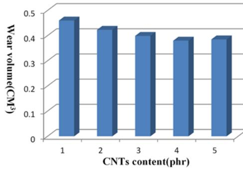
**Fig.3** Wear resistance of NR/CNTs nanocomposites
